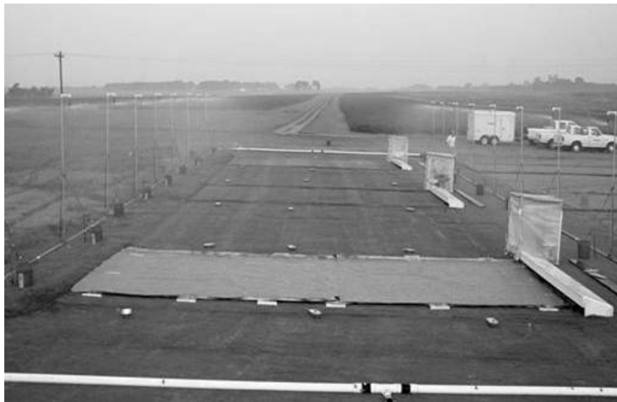
Figure 1. Co-verification of simulated rainfall application rate using rain gauges (metal pans) and a whole-plot plastic tarp (foreground).
