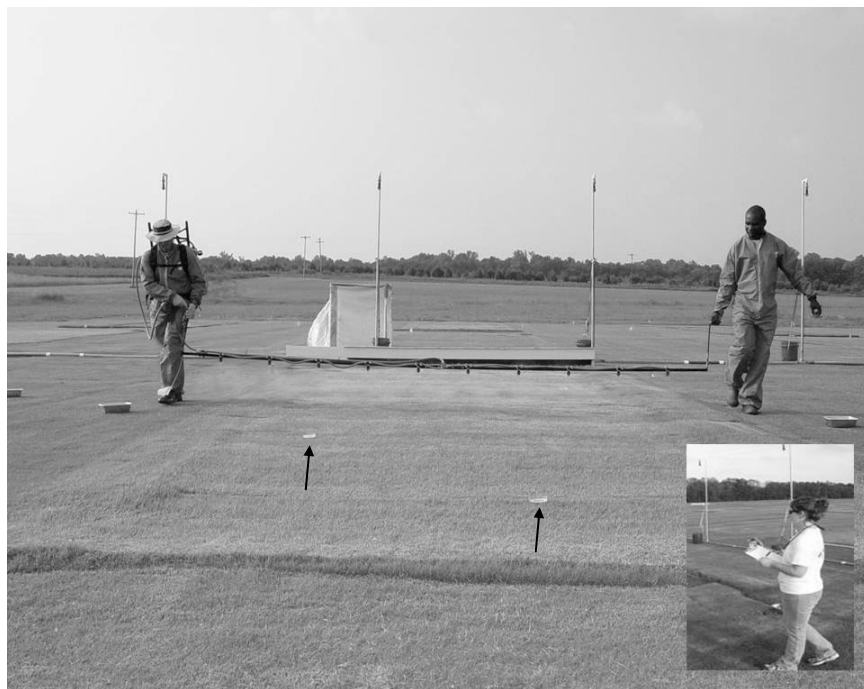
Figure 2. Co-verification of pesticide application rates using AV monitoring (Petri dishes, denoted by arrows) and pass-time methods (inset).
